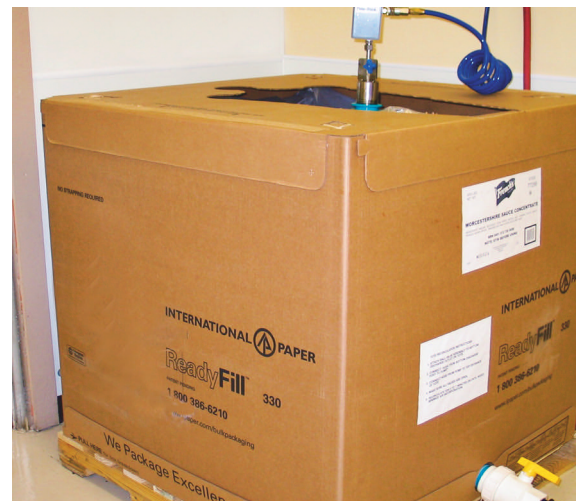
The 330-gal bag-lined tote is used to ship a secret liquid spice concentrate from French's Flavor Ingredients to Country Bob's facility, where the tote is used as a mixing vessel.
