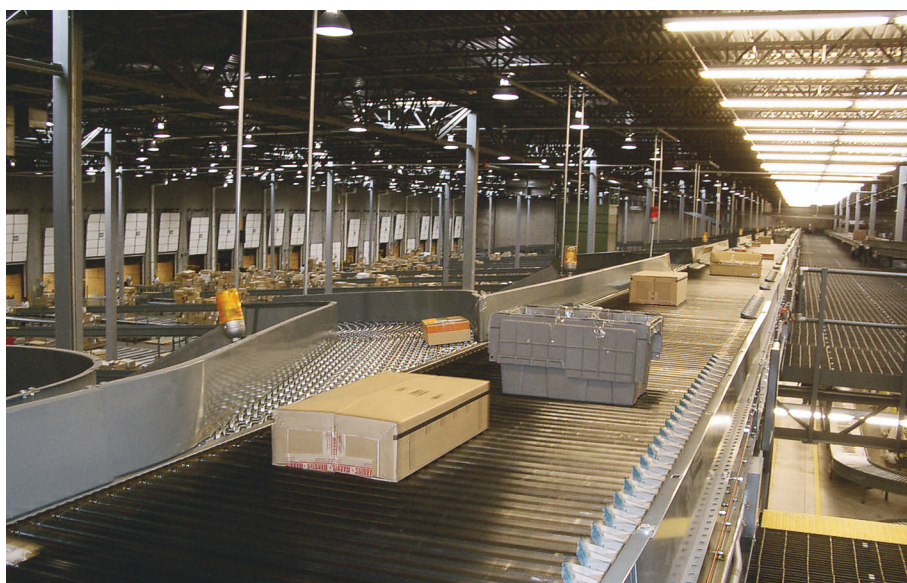
Two sliding shoe sorters offer throughputs of more than 250 cases/min, allowing Belk to keep a fast pace of items moving across the cross-docked warehouse.
