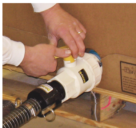
One side of the IBC has a ball valve on the bottom with a tapered sump to facilitate evacuation of the liquid concentrate blend.
