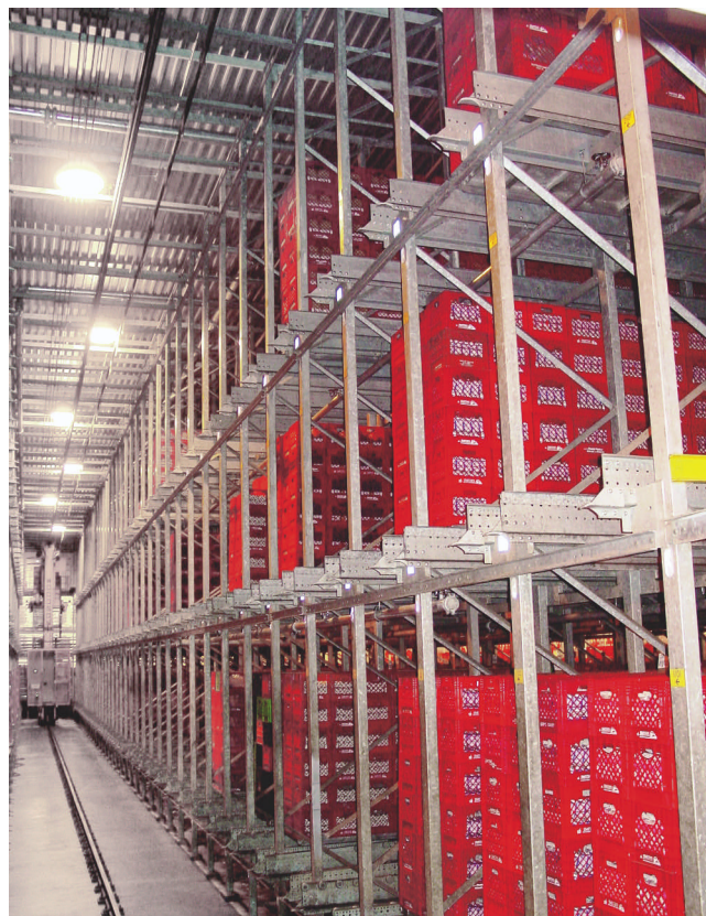
Medium-volume products are automatically palletized, and then placed by a crane into a high-rise storage system.
