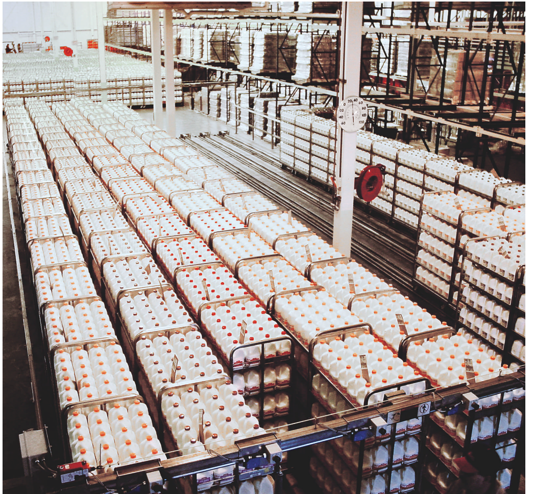
Bossy carts are either stored on the floor or are placed into 10 automatic storage lanes. The lanes move the carts forward to the unloading dock for picking an order.
