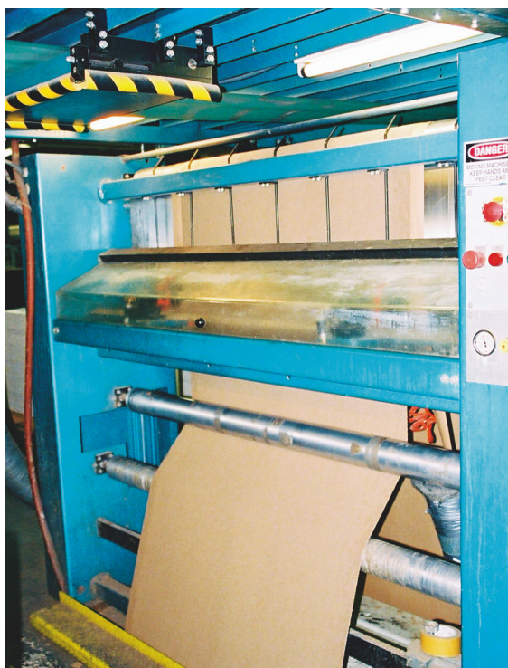
The single-face corrugated rollstock travels through the single-face laminator to be joined with the litho-printed label.
