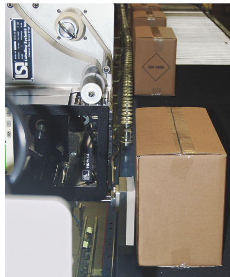
A narrow conveyor keeps cases gapped as they pass the printer/applicator for one to three labels.
