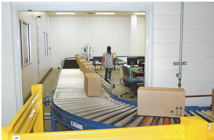
Turning through a portal on a 90-deg power-shaft conveyor, the cases feed to a skewed conveyor that shifts them to one side.
