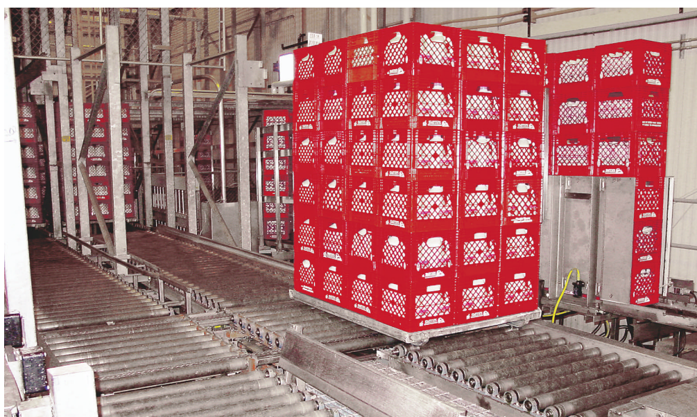
Pallet containing 12 6-high stacks is conveyed to the crane infeed, where it will be placed into storage.
