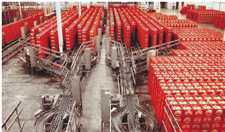
Two de-unitizers separate stacks of cases into a single file, after which the cases are conveyed to 16 high-volume accumulation conveyors for order picking.
